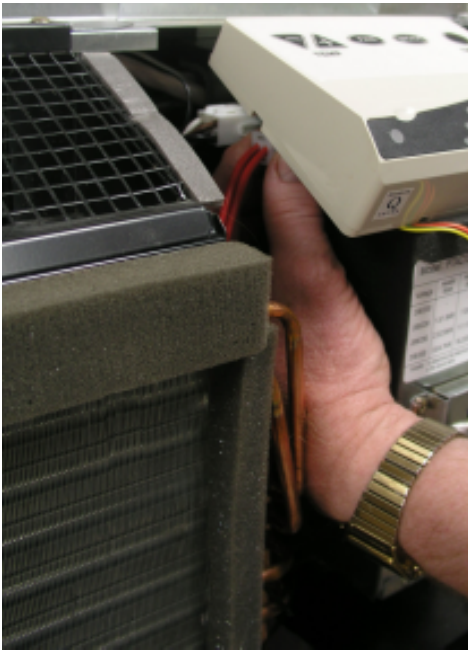
Figure 3. Reach Under the Control Pad, Squeeze the Latches on the Plug and Pull Loose from the Receptacle.
