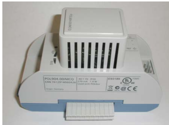
Figure 5. BACnet MSTP Communication Module with Board-to-Board Connector Inserted
