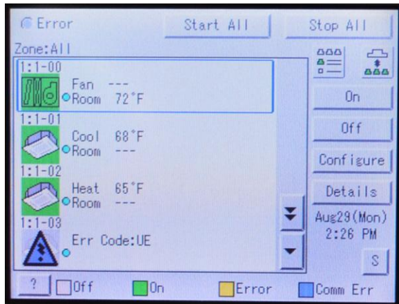
Figure 22, MicroTech III Air Handler in Unoccupied Operation
